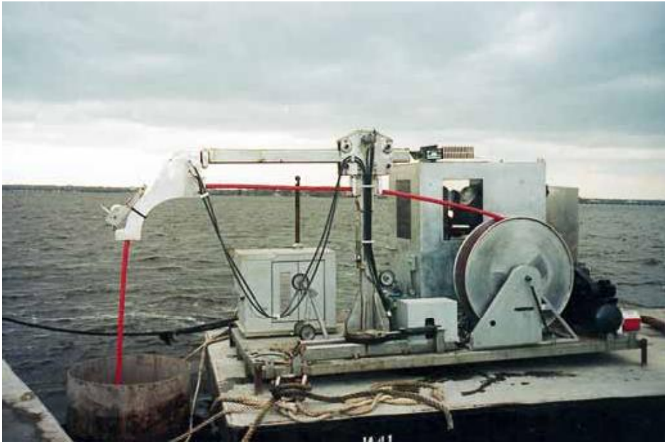
Figure 43, Shaft Inspection Device
