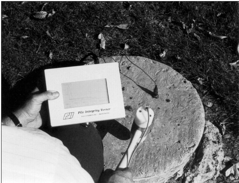
Figure 42, Pile Integrity Tester (After PDI, 1993)
